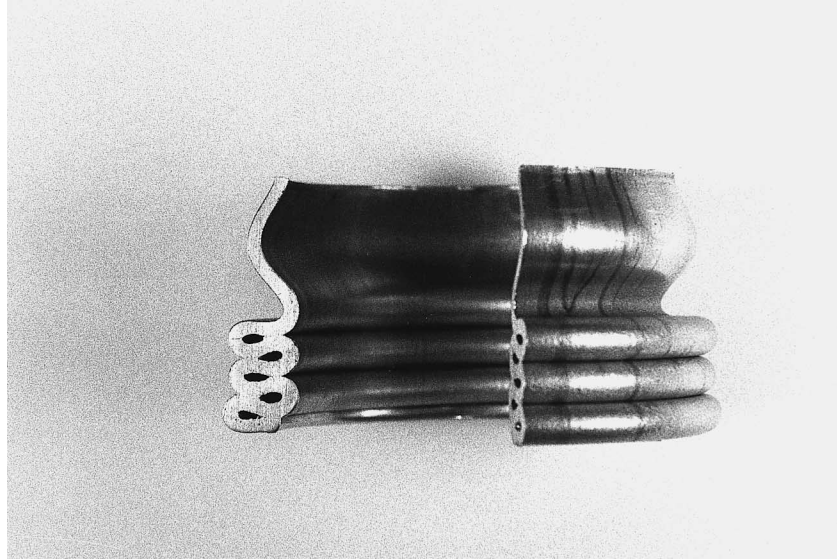
Fig. 2. Saw-cut through an axisymmetric collapsed thickwalled aluminium shell with R/h = 14 .
